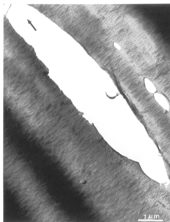
Figure 6. (a, Top) Electron diffraction pattern of a sheared film of polymer 1b . (b, Bottom) Electron micrograph of the sheared film of polymer 1b . The arrow indicates the shear direction.
