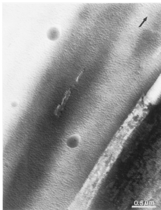
Figure 8. (a, Top) Electron diffraction pattern of a sheared film of polymer 3b . The arrow indicates the shear direction. (b, Bottom) Electron micrograph of the sheared film of polymer 3b . The arrow indicates the shear direction.
